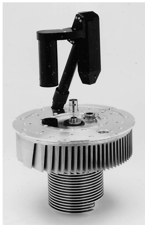
Fig. 1 The XL-I Optical System. The photograph shows the laser light source for the Rayleigh optical affixed to the "periscope", or toroidal diffraction grating which provides monochromatic light for the UV-visible absorption optics. Both systems are shown here mounted on the heat sink which normally resides beneath the floor of the centrifuge chamber
